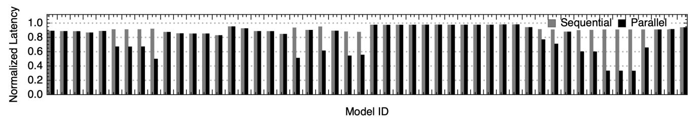
The sequential and parallel total layer latency normalized to the model's end-to-end latency using batch size 1 on c5.2xlarge
