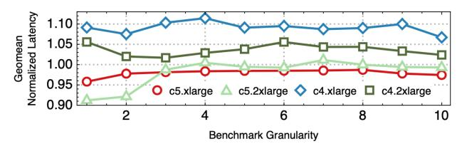
The geometric mean of the normalized latency (constructed vs end-to-end latency) with varying benchmark granularity from 1 to 10.
